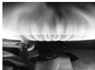
Proper burner and pilot burner pattern.
